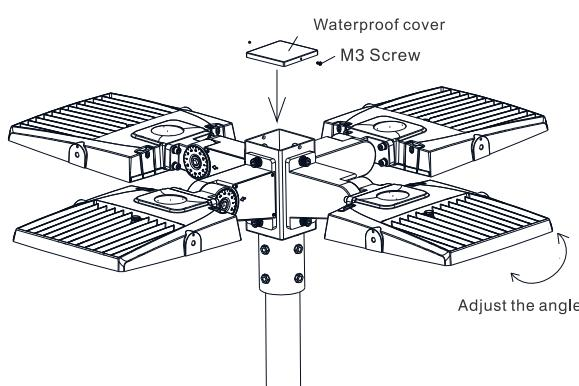
6. Install the waterproof cover onto the top of the adapter bracket and secure it with screws; Adjust the light output angle and fix the lamp to ensure reliable installation.
