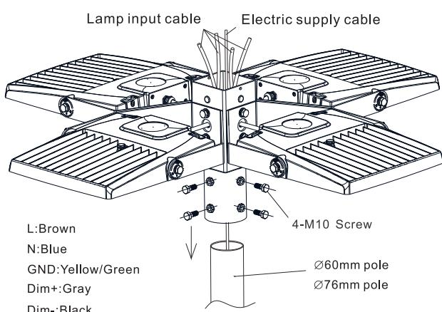
4. Use screws to securely fix the assembled lamp to the lamp pole; Each lamp's cable is connected in parallel with the mains cable and the wire ends are hidden inside the lamp pole.
