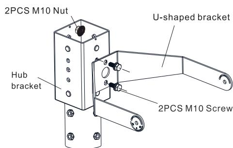
2. Connect the U-shaped bracket and the convert bracket with screws;
