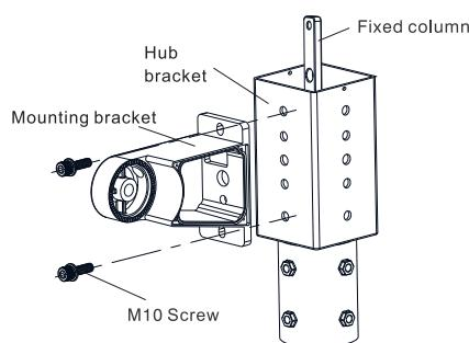
2. Secure bracket D to the hub using screws and nuts;
