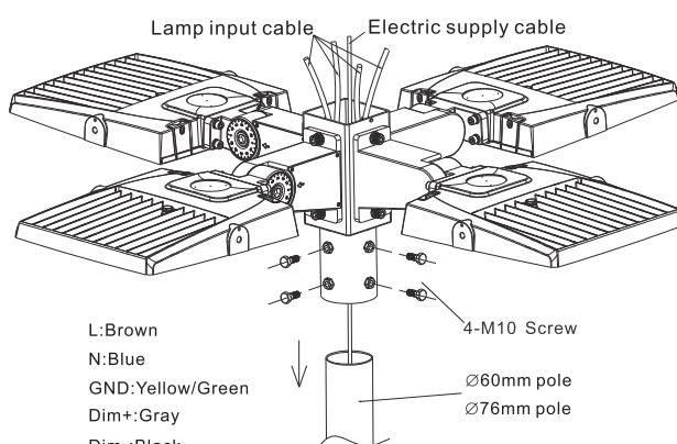
5. Use screws to securely fix the assembled lamp to the lamp pole; Each lamp's cable is connected in parallel with the mains cable and the wire ends are hidden inside the lamp pole;
