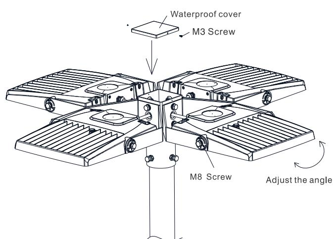
5. Install the waterproof cover onto the top of the adapter bracket and secure it with screws; Adjust the light output angle and fix the lamp to ensure reliable installation.
